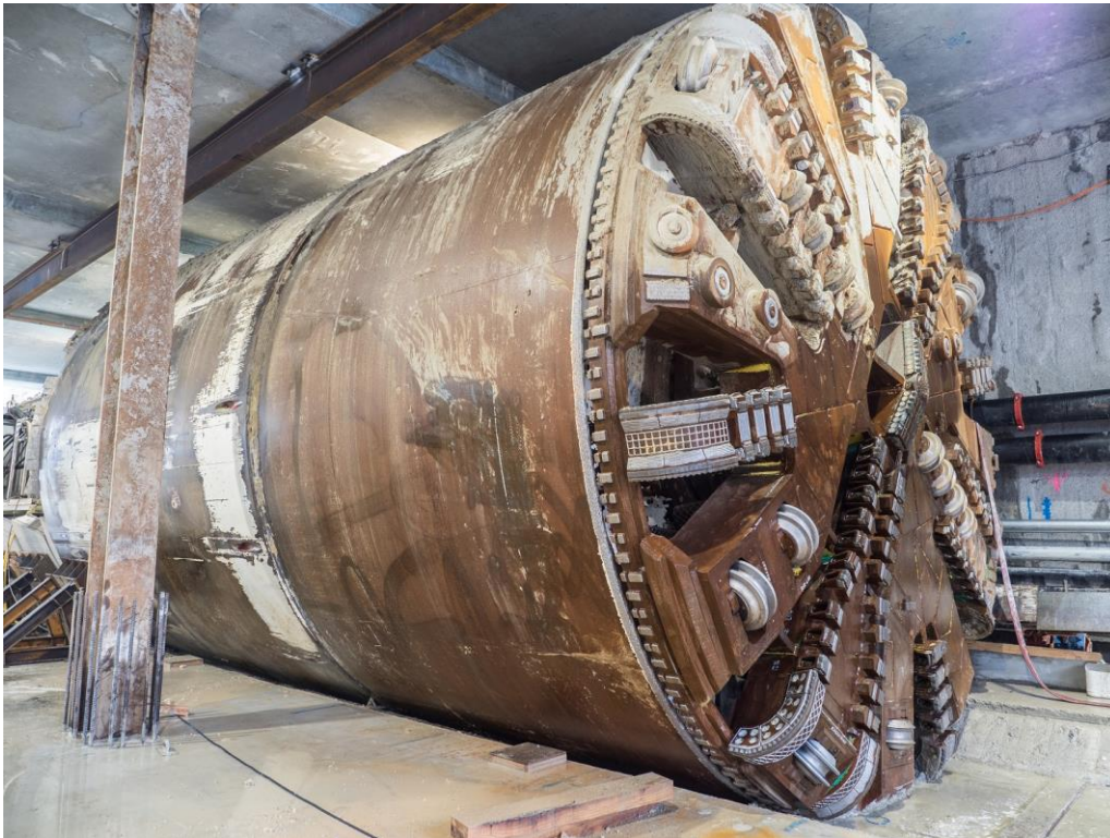
Figure 1 TBM used for tunnelling between High Wycombe and Bayswater
